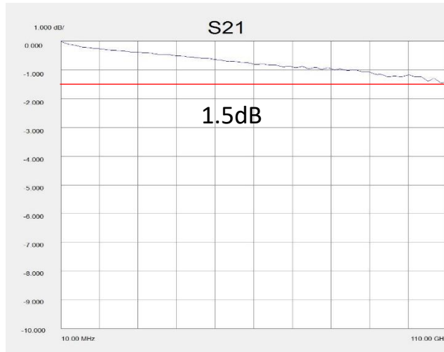
Typical Insertion Loss (GSGSG-150um pitch)
